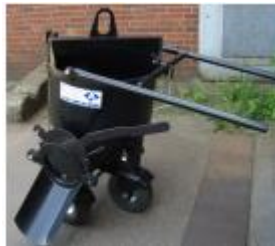
asphalt wheelbarrow huge version, round, none insulated , capacity appr. 100 litres, side outlet, 4 pneumatic tires, pushing handle swing over type, central crane hook
