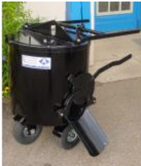
asphalt wheelbarrow huge version, round, insulated , capacity appr. 100 litres, side outlet, 4 pneumatic tires, pushing handle swing over type, central crane hook
