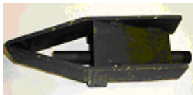
pulling shoe for wild cracks, to be fitted on a spraying lance
